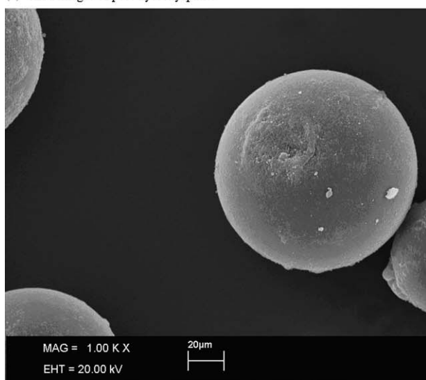
(b) SEM photographs of porous and spherical hydroxyapatite microcomposite
