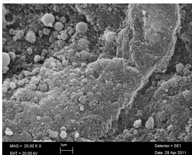
(c) Inside of crushed porous and spherical HA microcomposite
